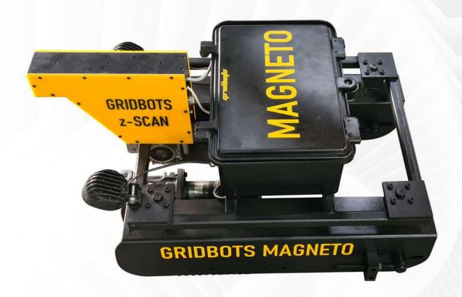
Gridbots Magneto series of robots are desgigned to be used in vertical and inclined waterwalls of powerplant boilers.
